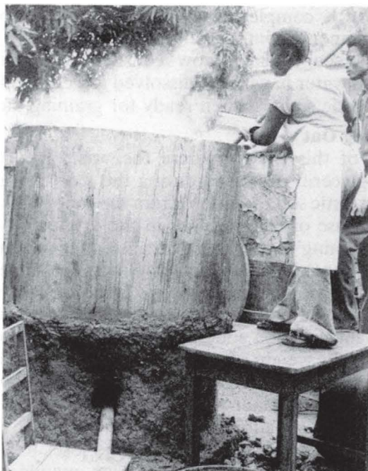
Plate 13: Soap-boiling using a TCC-designed boiling tank capable of producing 500 bars of soap a day
