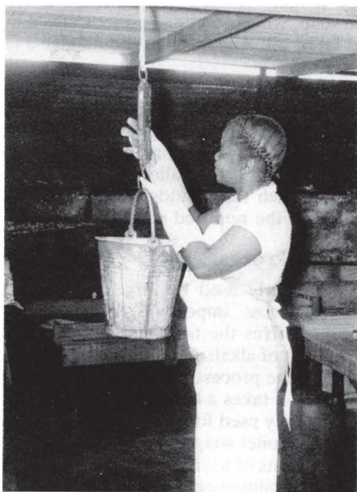
Plate 12: Weighing caustic soda with a spring balance
