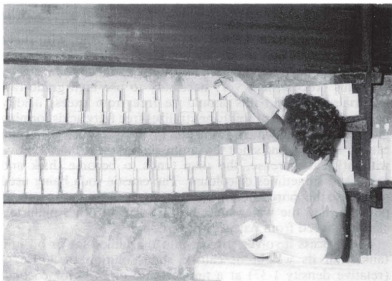
Plate 17: Arranging finished soap bars on shelves for drying
