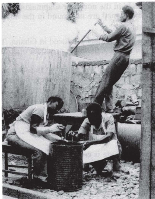
PLATE 4: Using hydrometer to determine the strength of caustic soda solution.
