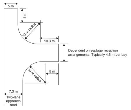
Figure 6.2 Typical tanker turning and discharge area layout
