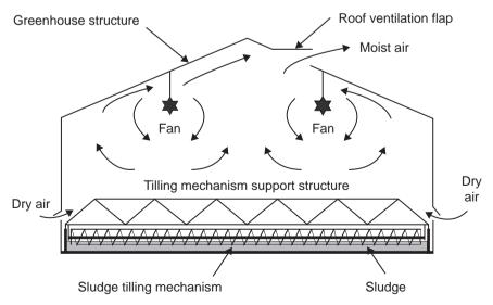
Figure 10.2 Solar drying in a greenhouse
