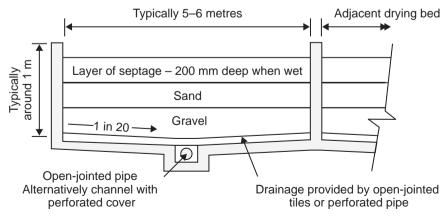
Figure 9.2 Cross-section of typical drying bed
