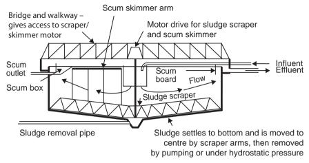
Figure 7.4 Conventional gravity thickener
