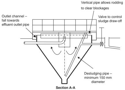
Figure 7.5 Plan and section of typical hopper-bottomed sedimentation tank
