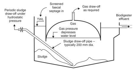
Figure 6.6 Section through fixed-dome biodigester
