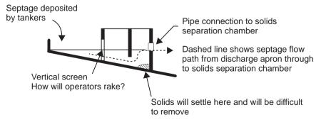
Figure 5.1 Inlet to SSC illustrating potential operational difficulties
