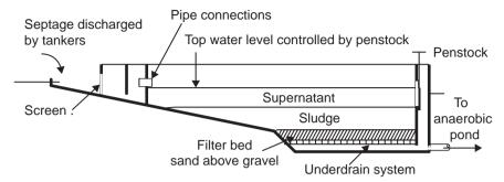
Figure 7.3 Longitudinal section through Tabanan solids separation chamber
