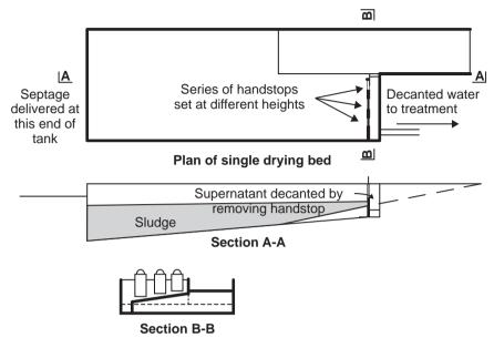
Figure 7.7 Possible shallow solids-liquid separation chamber arrangement
