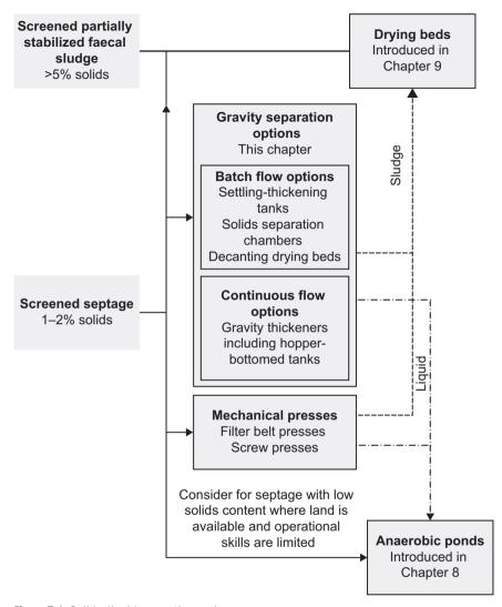
Figure 7.1 Solids-liquid separation options
