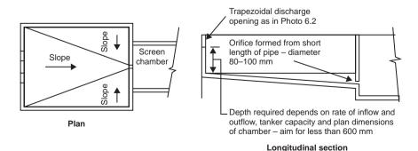
Figure 6.4 Simple arrangement for attenuating discharge flows
