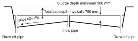
Figure 7.6 Section through decanting drying bed
