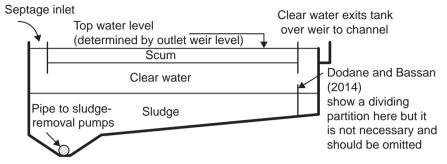
Figure 7.2 Longitudinal section through Dakar-style STT
