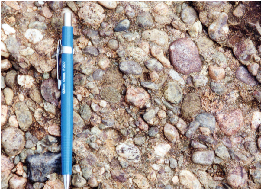
A32. Conglomerate: large pebbles cemented together in a finer grained matrix. BGS, © NERC 1999.
