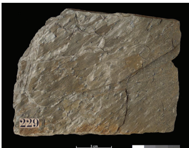
A39. Phyllitic pelite: metamorphosed mudstones and siltstones with shiny appearance from the mica and platy texture. BGS, © NERC 2002.
