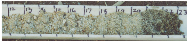
A8. Drill chips from a borehole drilled into granite: 0–3 m ferruginous soil; 3–4 m mottle clay; 4–11 m decomposed weathered granite; 11–21 m discoloured and broken granite; 21 m onwards unweathered fresh granite. BGS, © NERC 2000.
