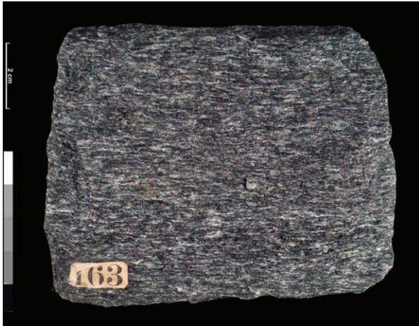
A42. Hornblende schist: metamorphosed mafic rich rocks (such as dolerite and basalt). BGS, © NERC 2002.
