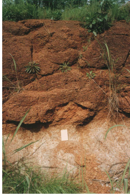
A2. Ferricrete: a hard red durable crust that can develop in tropical areas. BGS, © NERC 1998.
