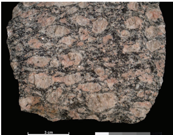
A44. Augen gneiss, characterised by large 'eyes' of lighter feldspar crystals. BGS, © NERC 2002.
