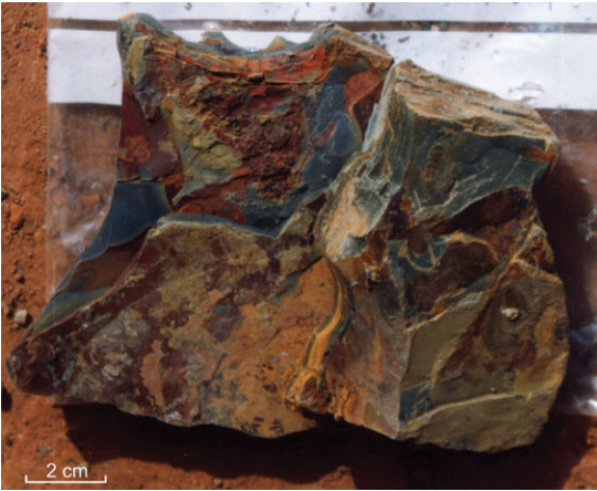
A33. A sample of weathered mudstone from a hand dug well stained by red/brown iron-oxides. BGS, © NERC 1999.
