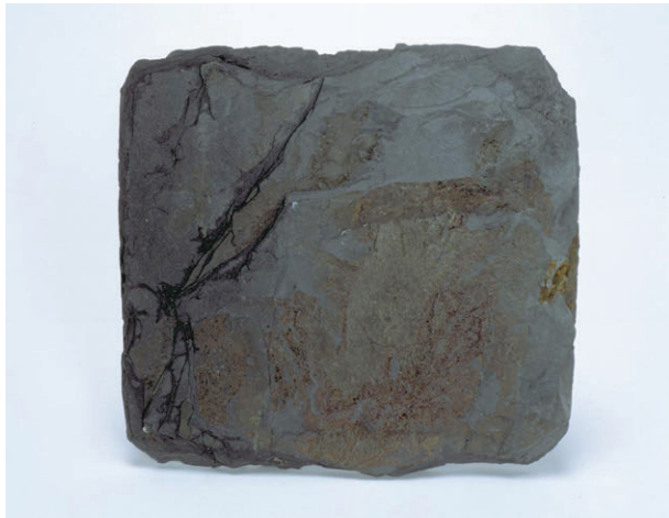
A40. Slate (phyllitic pelite): metamorphosed mudstone which can easily split along parallel planes. BGS, © NERC 2002.
