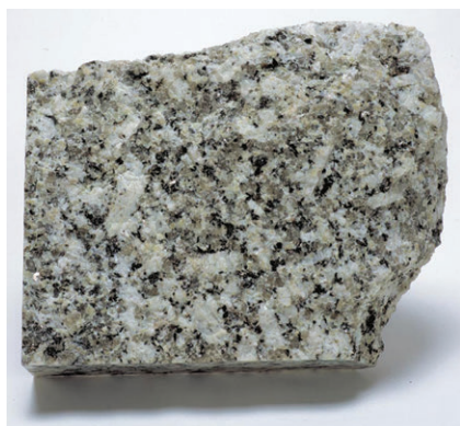
A11. A grey granite composed of grey quartz, white feldspar and black mafic minerals. BGS, © NERC 2002.
