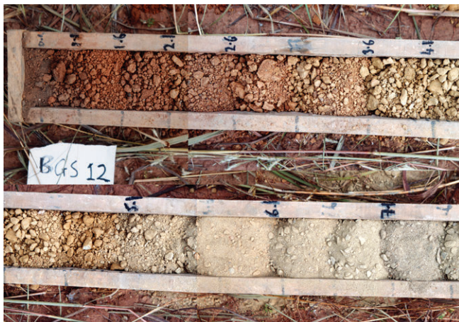
A8. Drill chips from a borehole drilled into granite: 0–3 m ferruginous soil; 3–4 m mottle clay; 4–11 m decomposed weathered granite; 11–21 m discoloured and broken granite; 21 m onwards unweathered fresh granite. BGS, © NERC 2000.
