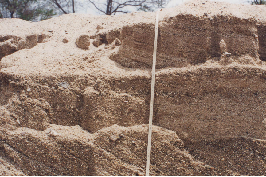
A5. Cross bedded unconsolidated sands exposed in a trench in Botswana. BGS, © NERC 1998.
