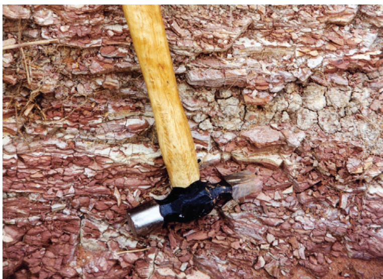
A34. Weathered red mudstones exposed in a river bank. BGS, © NERC 1999
