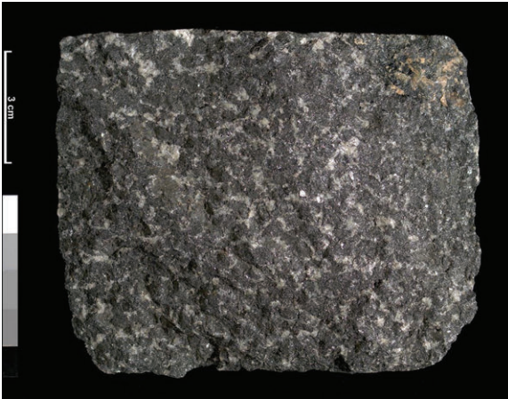
A17. Dolerite: medium grained igneous rock dominated by black mafic minerals. BGS, © NERC 2002.
