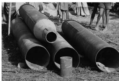
Mild steel casing with a reducer
