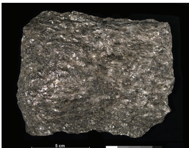
A41. A schistose pelite: metamorphosed mudstone and siltstones with a characteristic shiny appearance from the mica. BGS, © NERC 2002.
