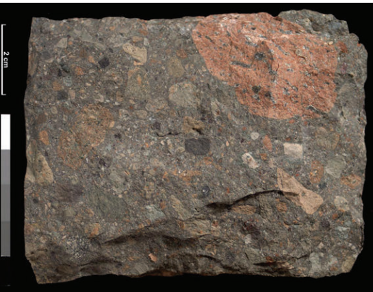
A24. A pyroclastic rock composed of large rock fragments set in a fine matrix of volcanic ash. BGS, © NERC 2002.
