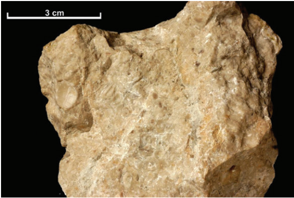
A36. A pale coloured limestone containing fossils. BGS, © NERC 2002.
