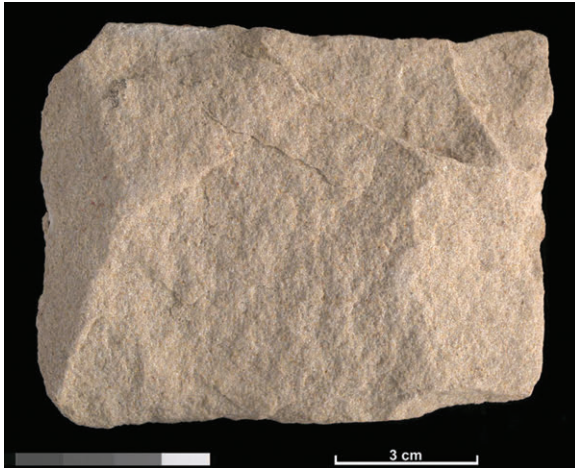
A26. Fine to medium-grained well sorted quartz sandstone. BGS, © NERC 2002.
