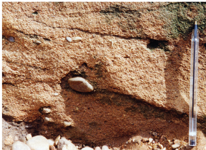
A28. Coarse-grained, pebbly sandstone. BGS, © NERC 1999.
