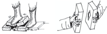
Figure 40: Brick test: resist 3 point test and give a ringing sound when struck together
