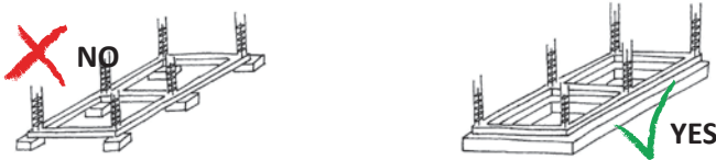
Figure 83: Foundations must be continuous to support the walls on their whole length
