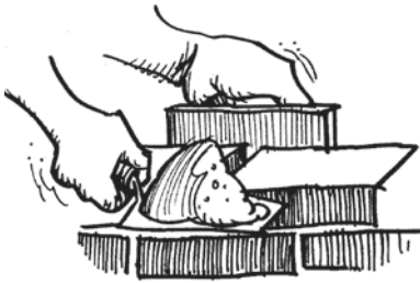
Figures 131: Placing the mortar and bricks
