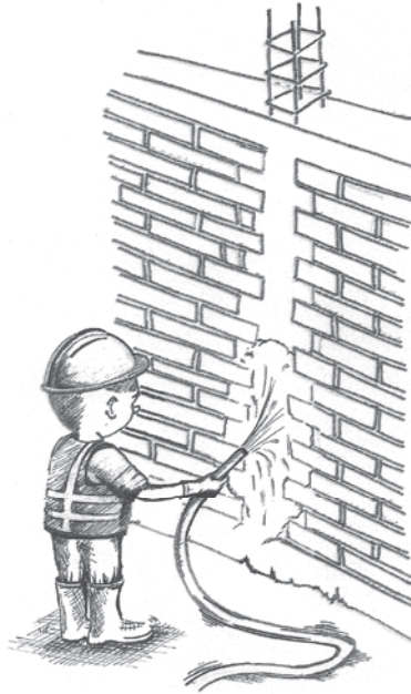
Figure 145: Water concrete 3 times a day for 7 days
