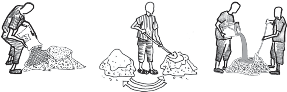
Figure 56: Hand mixing of concrete, from left to right: first dry mix twice, then add water
