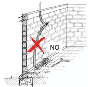
Figure 135: Never break up the walls for conduits
