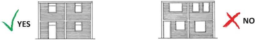
Figure 32 a): Windows should be placed in the same position on each floor
