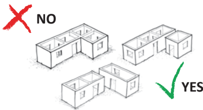
Figure 18: Buildings with complex forms should be divided into several independent simple forms
