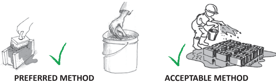
Figure 67: Drenching masonry units before use is very important
