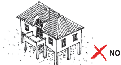
Figure 25: Never place a building on columns
