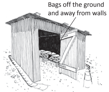
Figure 45b: Keep cement in a dry shed
