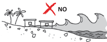
Figure 11: Don't build too near the sea: storms or tsunamis can flood the area
