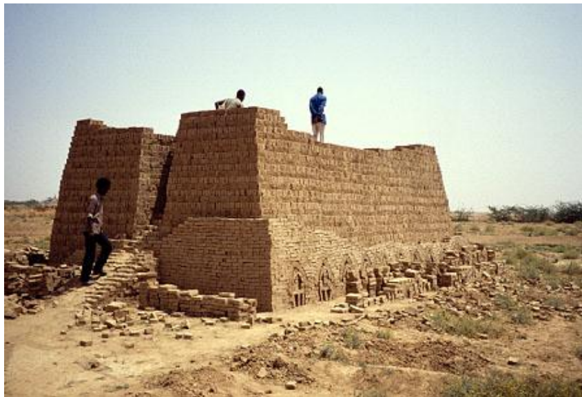
Figure 1: Large clamp kiln near Kassala, Sudan. ©Practical Action/Theo Schilderman
