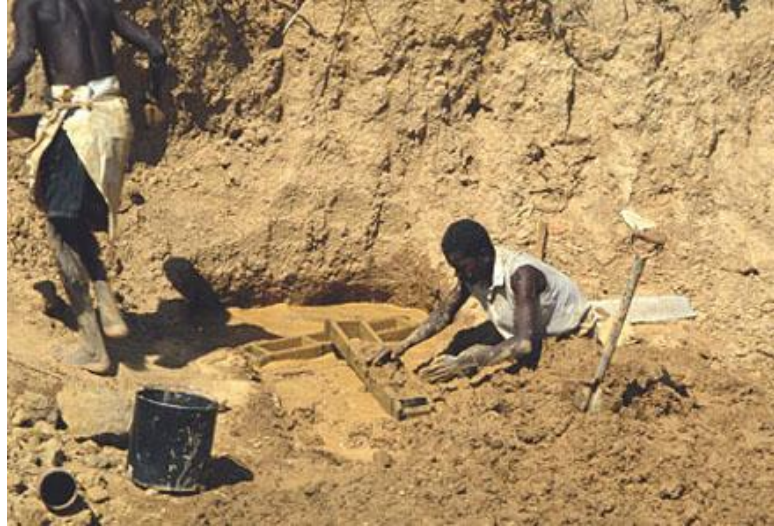
Figure 2: Slopmaking in a triple mould, Zimbabwe. ©Practical Action/Theo Schilderman
