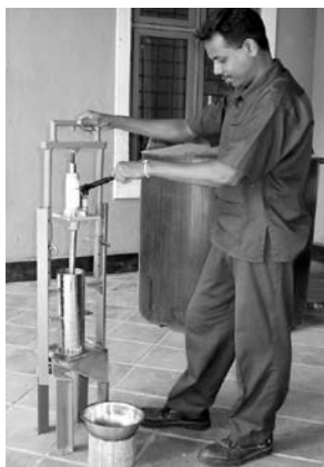
Photo 30 oil separation using press equipment
