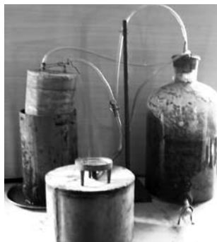
Photo 35 Lab scale bio gas unit – 10 litre aspirator bottle capacity, NERDC developed small biogas burner, neem residue and straw raw material
