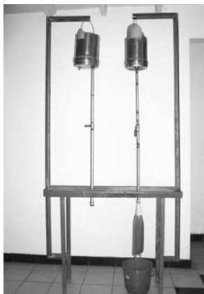
Photo 28 Gravity type oil filter
