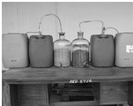
Photo 34 Press residues are ready for initial biogas bottle testing
