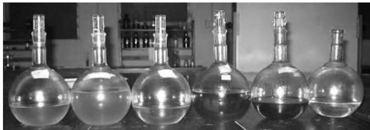
Photo 41 Biodiesel samples processed at the CPE laboratory (from left to right: jatropha, castor, rubber, neem, domba and coconut)
