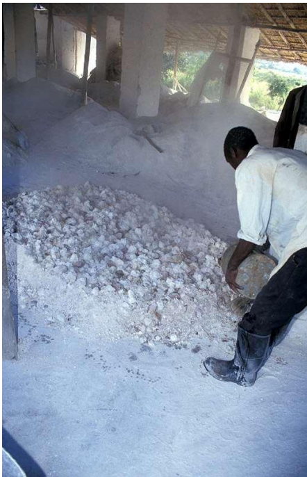
Figure 3: Hydrating of quicklime using a watering can Chenkumbi Limeworks, Malawi. Photo: Practical Action / Dave Mather.
