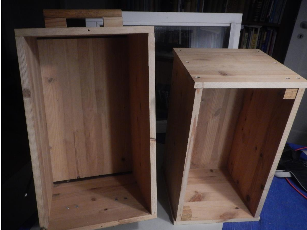
Fig. 1. The solar oven. Front left: The outer box. Front right: The inner box. Behind: The window.
