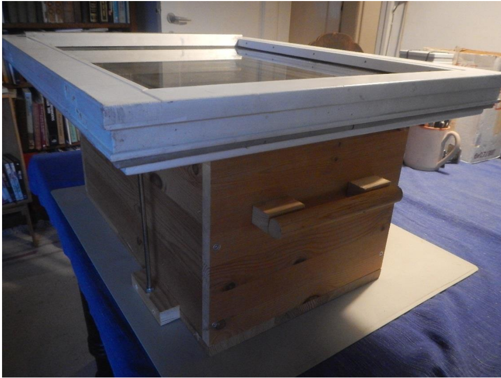
Fig. 4 shows the A version of the solar oven, where the window overhangs the sides of the outer box.
