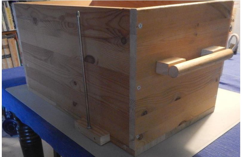
Fig.11. The rod to assist the inclination and the direction of the solar oven.
