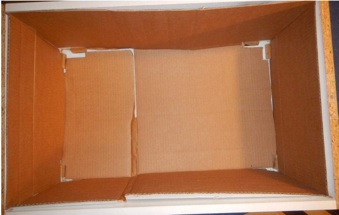
Fig. 6. Insulation: 2.5 mm cardboard.
