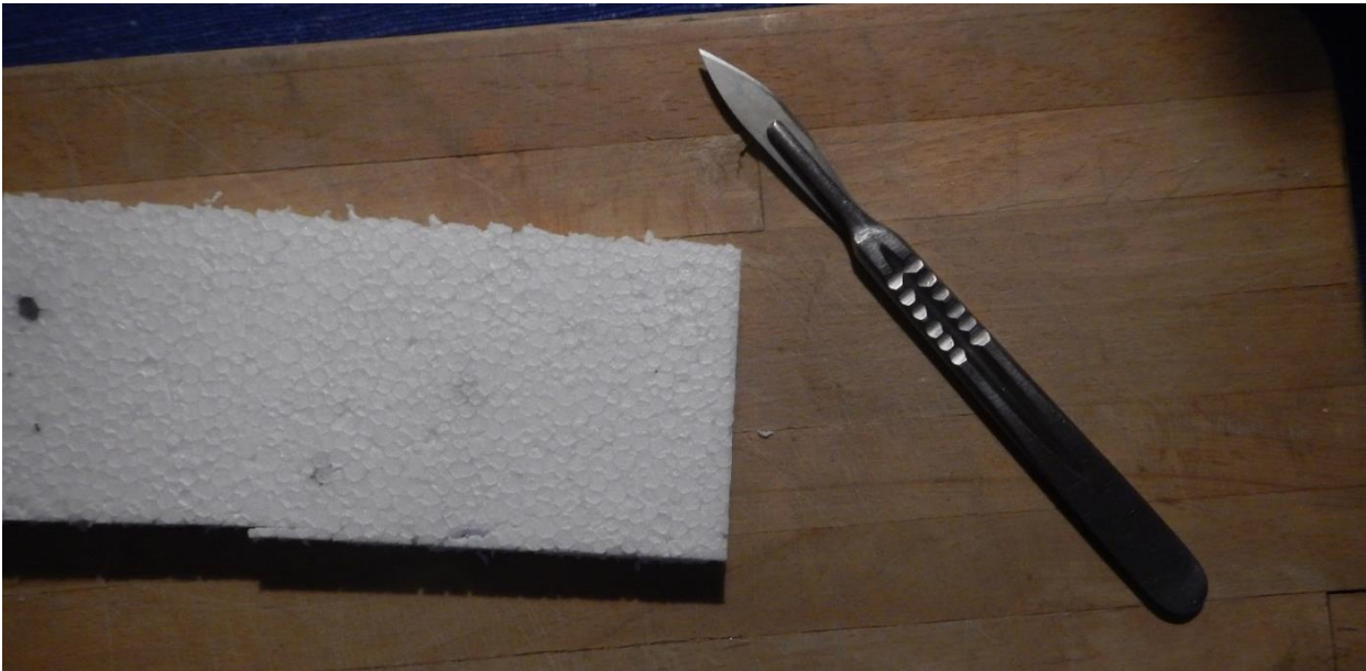
Fig. 12. Insulation material: Polystyrene Thickness 10 mm. A scalpel and a breadboard were used for the sizing.
