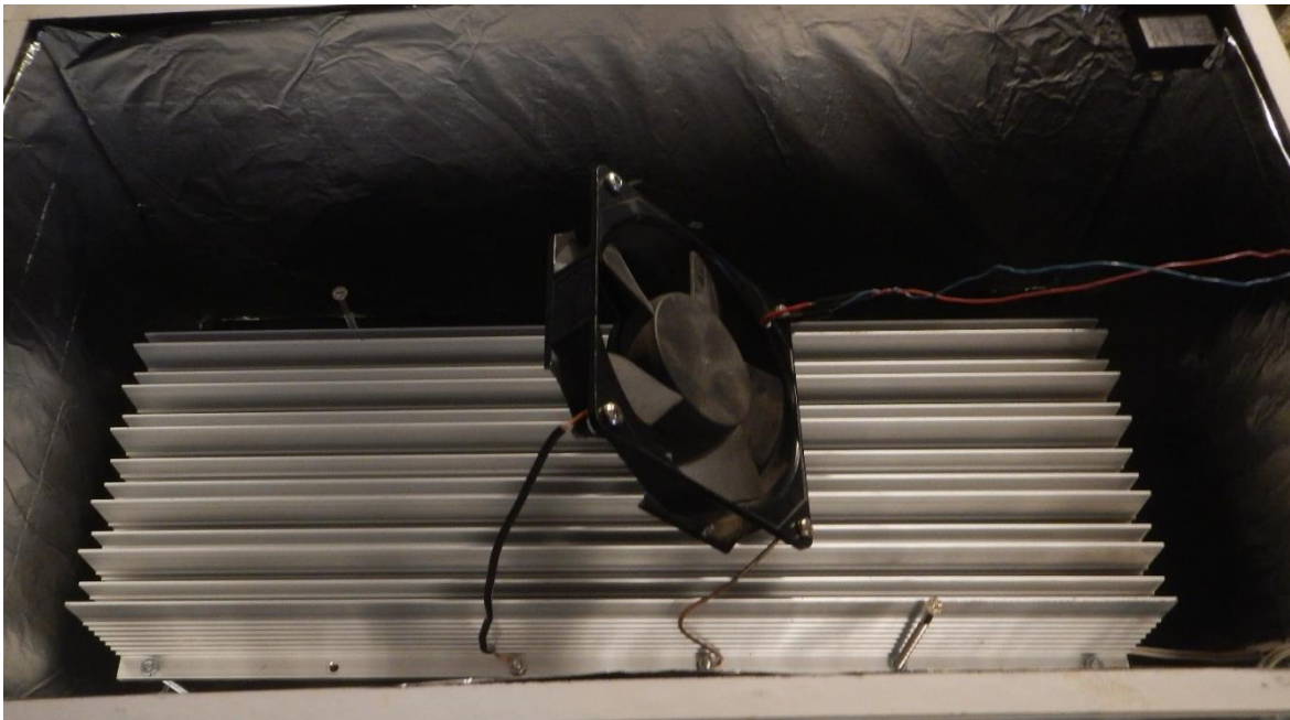
Fig. 3. The heatsink resting on 30 mm 4M screws at the bottom of the oven. Power supplied by red, blue and grey wires. The two aligned 5.0 mm holes in the end of the inner box and the end of the outer box accommodated: A. The two 1.65 mm \varnothing wires to the three 75 \Omega / 50 W power resistors - and B. The two 0.9 mm \varnothing wires to the fan. C. Finally, the 2.0 mm \varnothing wire for the thermometer was also fitted in.
