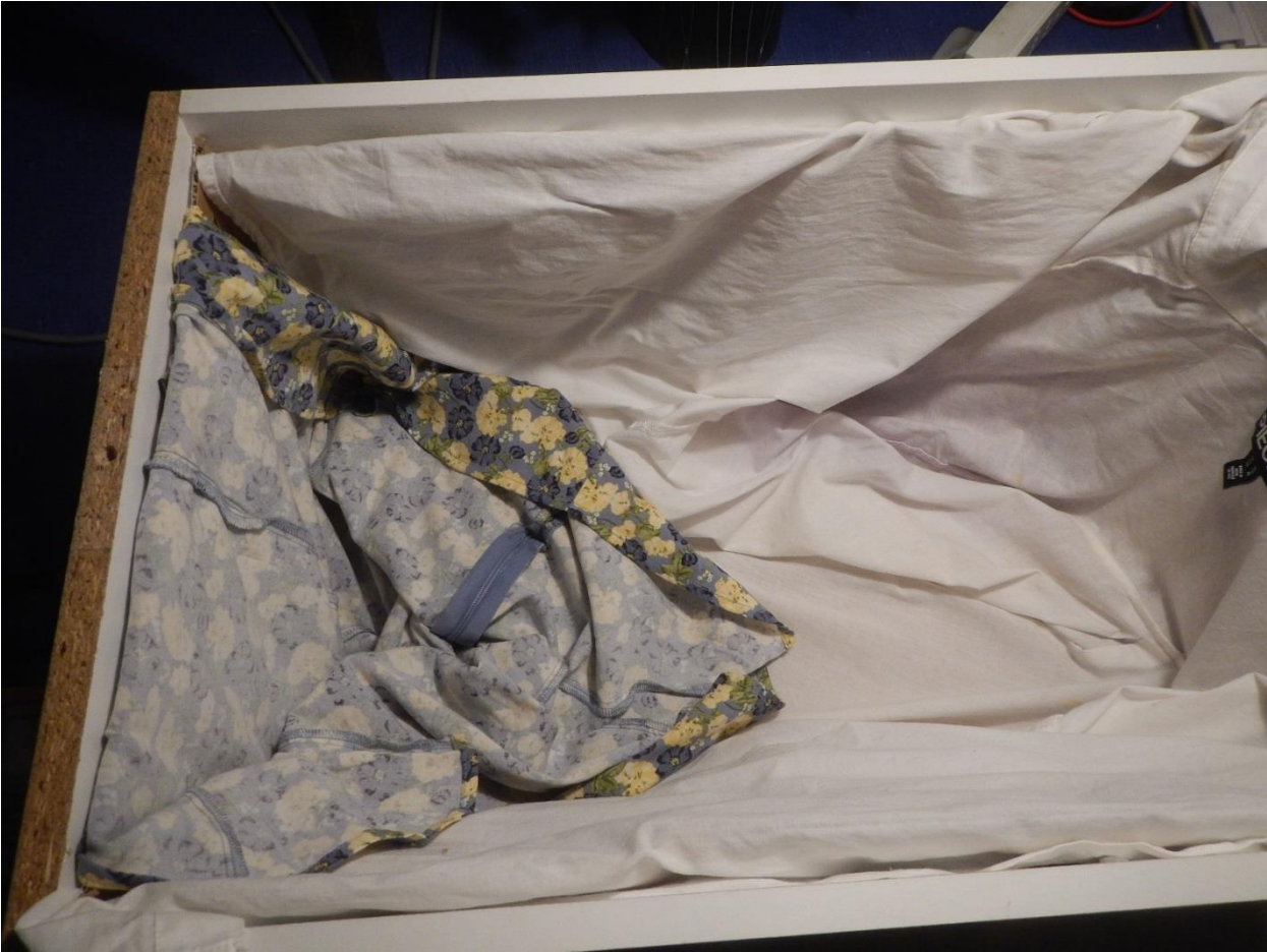
Fig. 11. Insulation material: Thin fabrics - in form of a shirt and a skirt suspended on cardboard.
