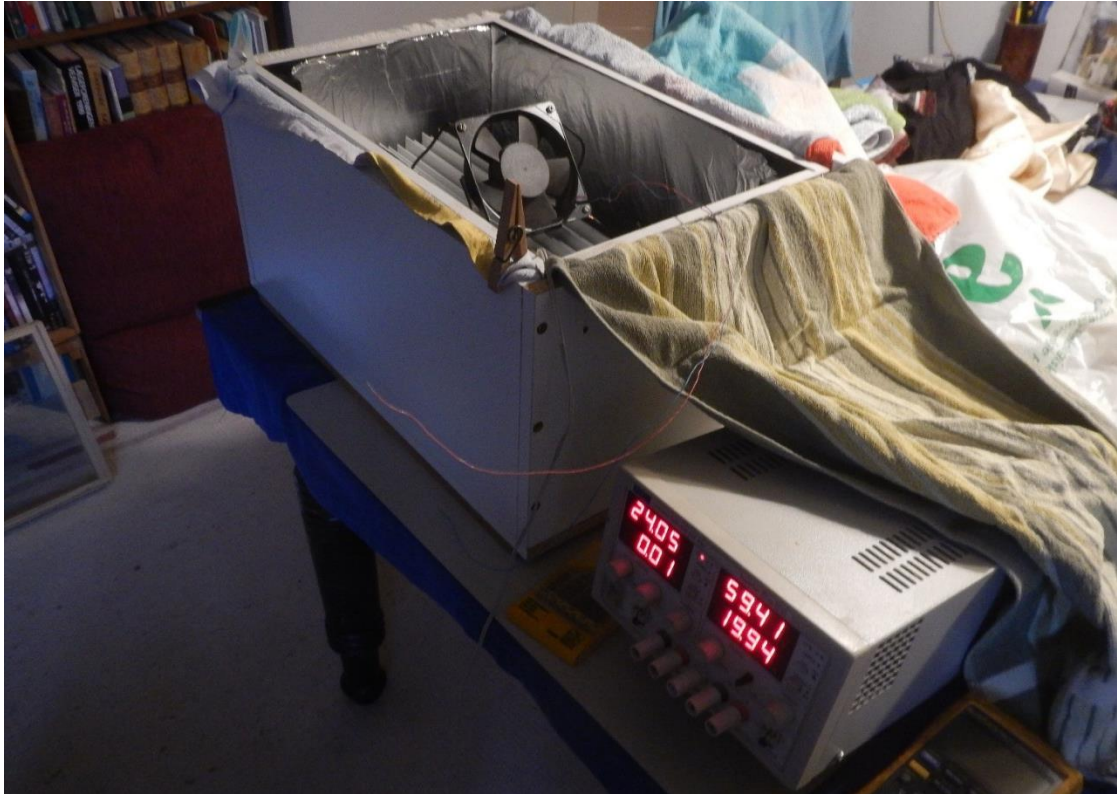
Fig. 5. Insulation material: Two towels. Left: solar oven, middle: Power supply (24 V and 59.4 V) right: multimeter.
