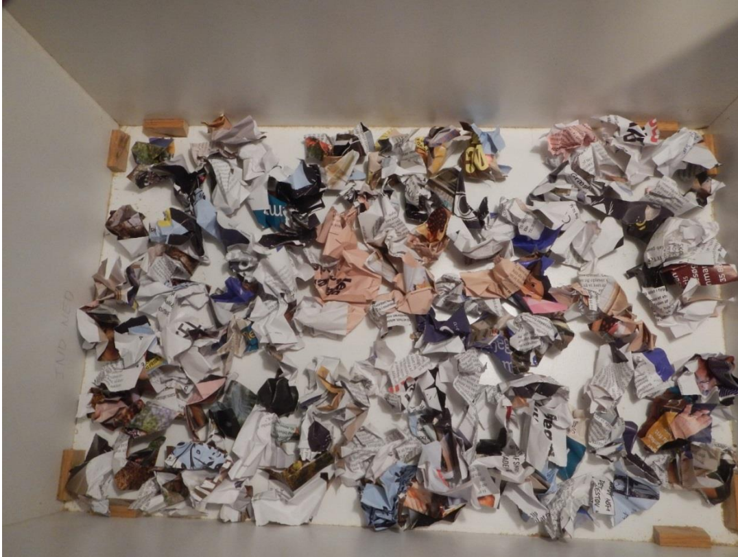
Fig. 7. Insulation: Hand curled paper balls.
