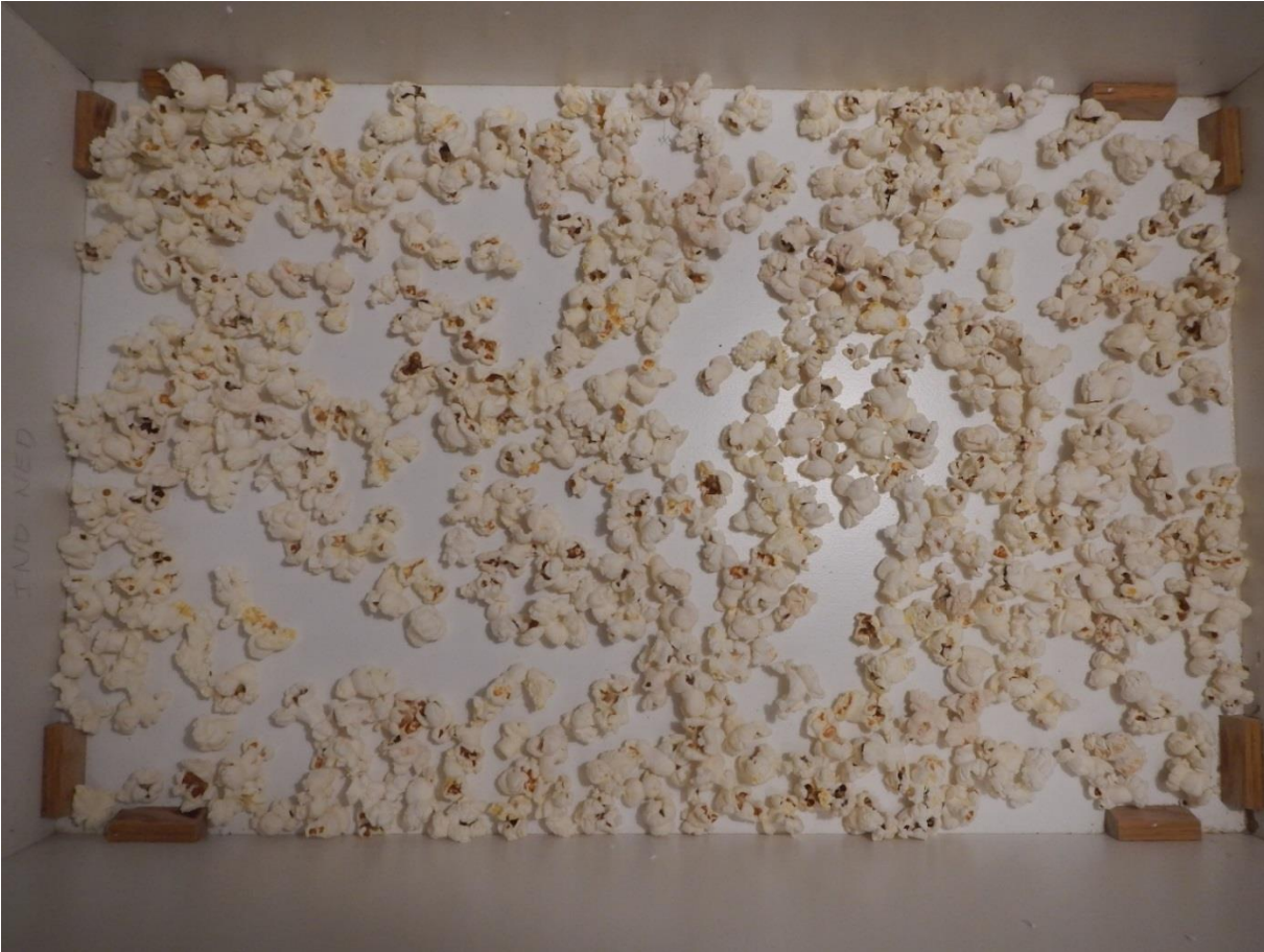
Fig. 13. Insulation material: Popcorn.
