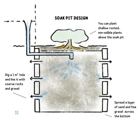
The anal cleansing water can be piped outside the toilet to a soak pit. If this is not possible, the water can be collected in a jerry can and emptied into a pit latrine or foul water drain if the household are willing to manage this.
