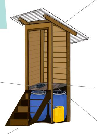
WATERPROOF ROOFING SHEET Corrugated steel or thatch panels, felted timber sheet or UPVC
