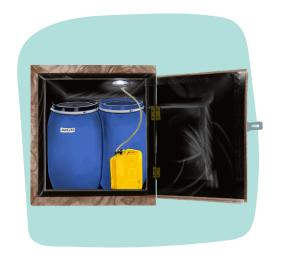
Open the chamber under the toilet and put on the lid of the barrel.
