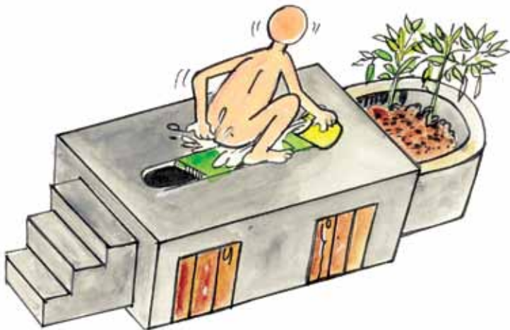
Double chamber, squatting, outside, washes without urine collection.
