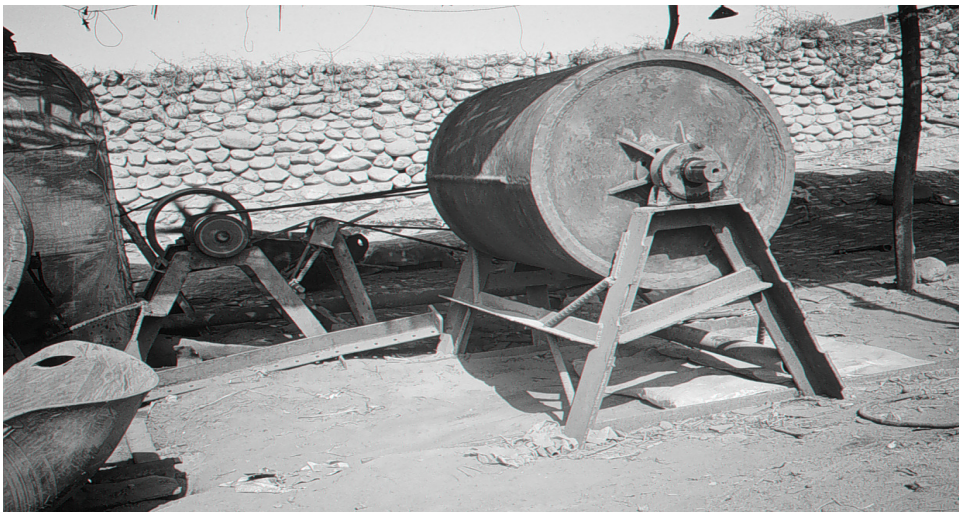
Figure 3: A ball mill being used as part of a gold mining operation in Arequipa, Peru ©Practical Action
