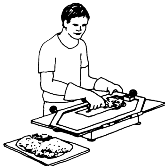
Figure 2: Work the mortar mix under vibration
