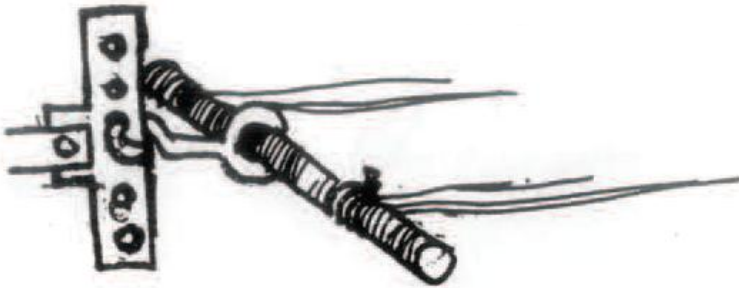
4.3. When the donkey is tired and soil humidity is low the hook should be connected to the lowest hole.
