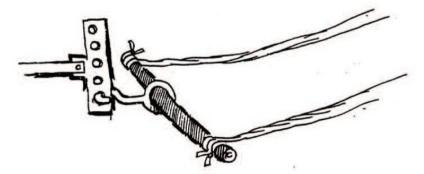
Control of the plough adjustment can be obtained by either increasing or decreasing the rope length between the plough and donkey or by moving the main bar upward or downwards.
