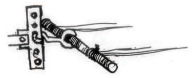
4.3. When the donkey is tired and soil humidity is low the hook should be connected to the lowest hole.
