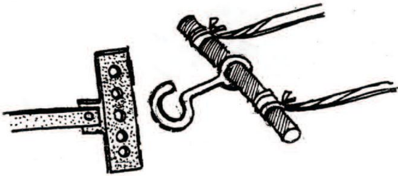
4.1. The hook is connected to the hole furthest along the bar if deep ploughing is required.
