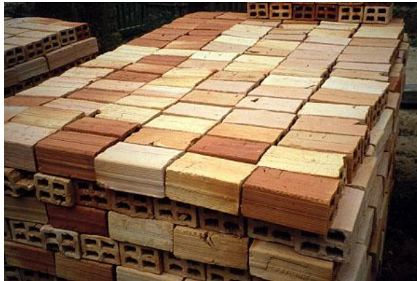
Figure 2: A pile of fired bricks, Alto Mayo, Peru. To be noted are the cracks and deficiencies in the bricks. Photo: Practical Action / Theo Schilderman.
