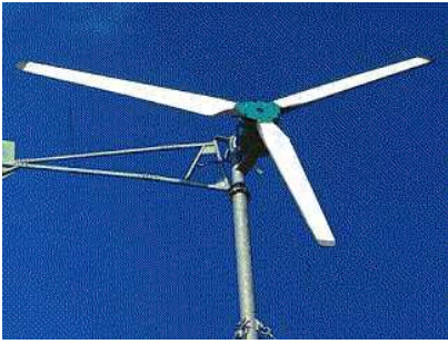
Figure 1: Low solidity rotor Photo: Practical Action
