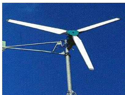
Figure 1: Low solidity rotor Photo: Practical Action
