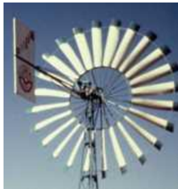
Figure 2: High solidity rotor Photo: Practical Action
