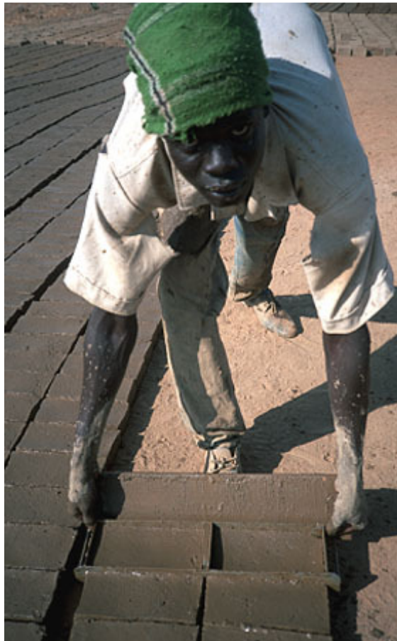
Figure 3: Brick-making using improved kiln at Kassala, Eastern Sudan. Releasing the moulds and laying bricks for drying. Photo: Practical Action / Mohammed Majzoub.
