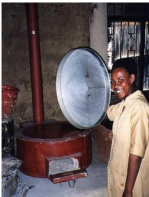
Figure 7: Commercial Mirte stove (photo: ESD)
