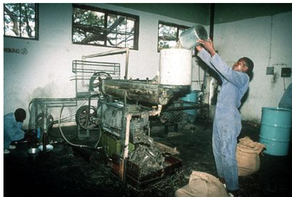
Figure 5: Tinytech oil expeller in operation in Zimbabwe.
