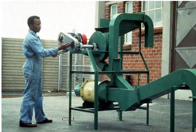
Figure 3 : Decortication (removal/winnowing of husks) machine for sunflower seeds. The decortication machine is used in conjunction with Tinytech oil mills. Photo credit: Kieth Machell / Practical Action
