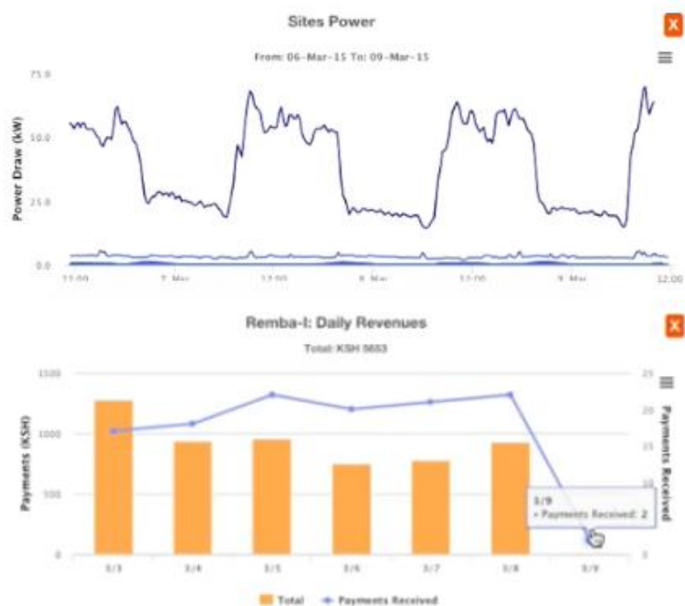
Figure 5: Real-time performance monitoring of a SteamaCo micro-grid in Kenya on their Dashboard.
