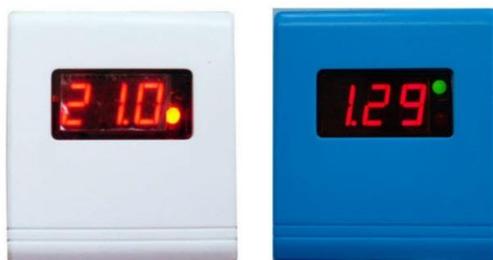
Figure 5: Electricity load limiter by Shenzhen Sailwider Electronics Co., Ltd. The limiter automatically gives an alarm or cuts off the power supply when the electrical power consumption is higher than a pre-set value.
