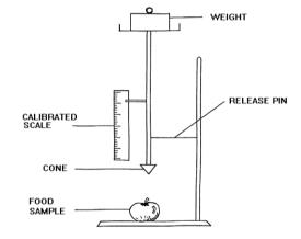
Figure 1: Fruit hardness test using a penetrometer.
