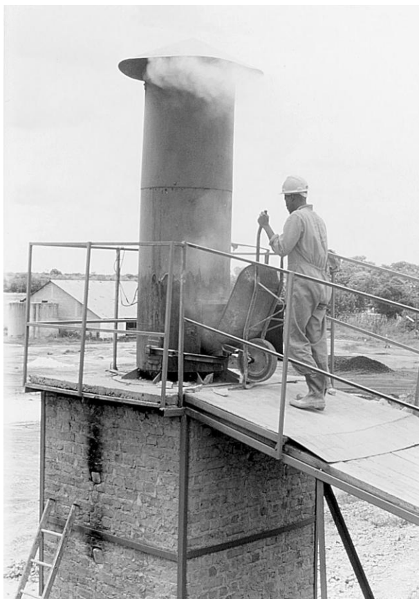
Figure 1: Loading stone/fuel through the hopper at the chimney level, lime kiln, Chegutu, Zimbabwe Photo: Practical Action / Kelvin Mason.
