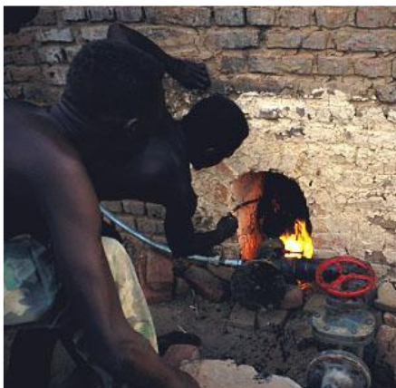
Figure 1: Brickmaker lighting a kiln with a liquid fuel burner. Photo:
