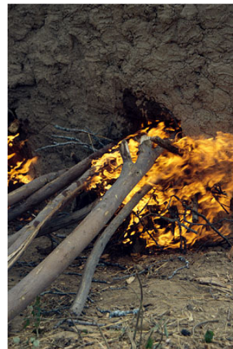
Figure 2: Firing bricks using wood as a fuel. Photo: Practical Action.
