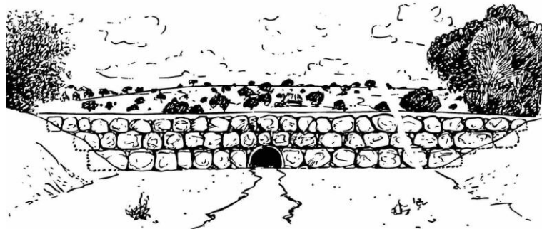
Figure 6: Tying in the ends of the bank
