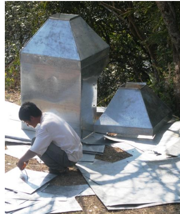
Figure 5: Manufacturing a smoke hood using hand tool in Nepal.
