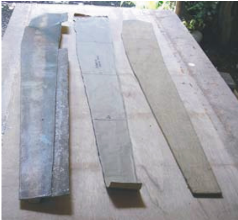
WINDWARD MOULD PAPER TEMPLATE PLYWOOD TEMPLATE
