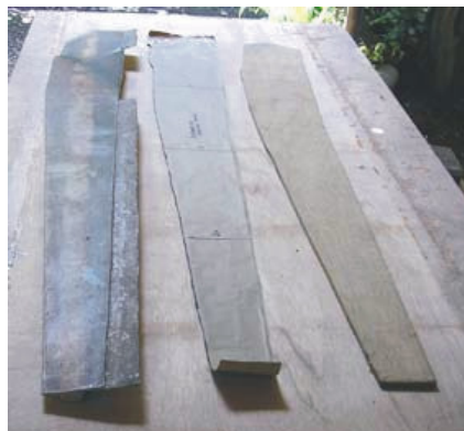
WINDWARD MOULD PAPER TEMPLATE PLYWOOD TEMPLATE
