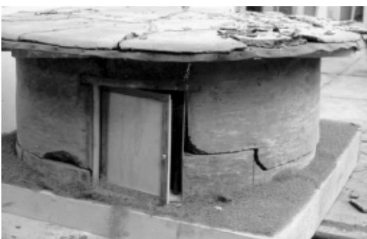
3-4 to 3-8 Earthquake tests with models of square and circular shape (Minke 2001)
