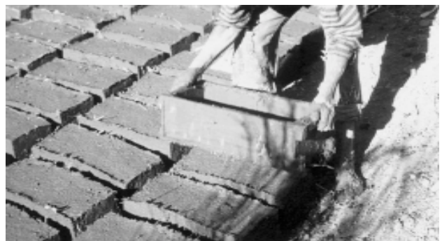
7-2 Production of adobes in Ecuador
