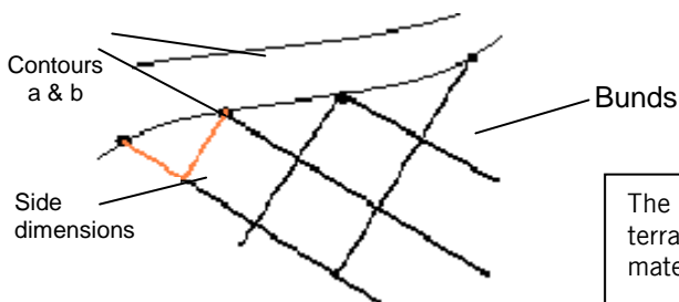
Figure 6: Laying out the bunds using contours
