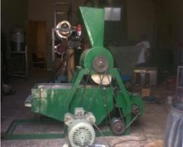
Figure 5. Completed millet thresher and cleaner.
