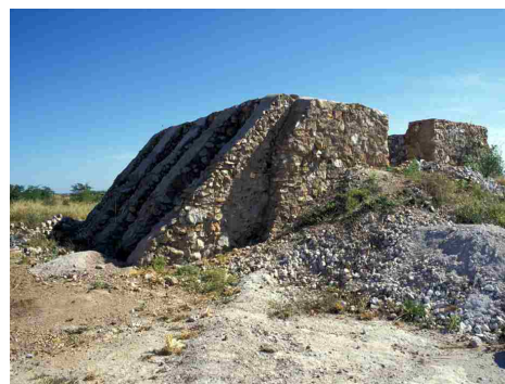
Figure 2: Malawian box kiln Photo credit: Practical Action/Kelvin Mason
