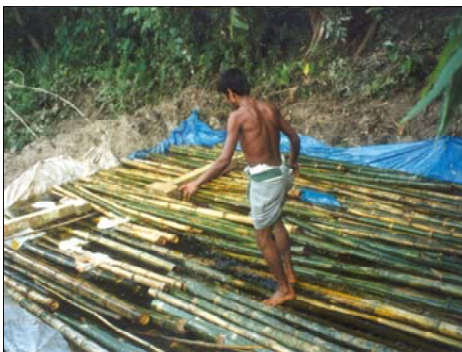
Figure 4: Curing bamboo trees for building flood resistant houses Faridpur, Bangladesh. Photo: Practical Action Bangladesh.
