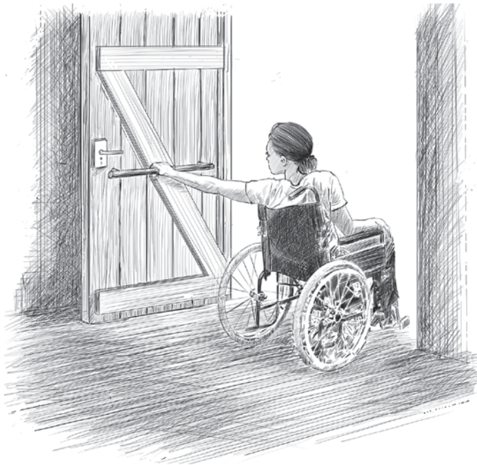
Figure 5.5 Handle extended to full width of door Source: Adapted from (** Jones & Reed, 2005)
