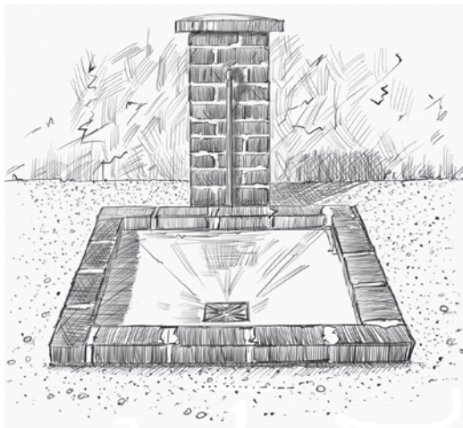
Figure 12.2 Simple sluice for disposal of faeces
