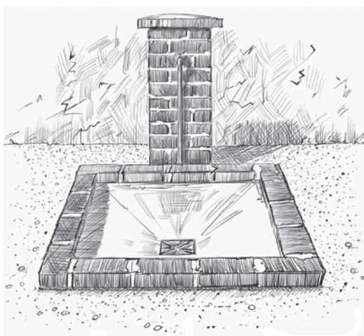
Figure 12.2 Simple sluice for disposal of faeces
