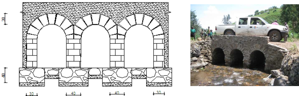
Fig. 18: Multiple stone arch culvert- - dimensions in cm.
