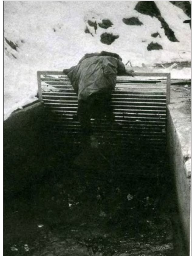
Photo 5.11 Cleaning can be difficult with horizontal bars
