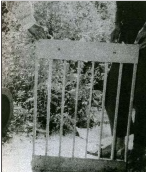
Photo 3.4 Coarse trashrack for 50 kw Galkot MHP, Baglung, Nepal. 65 mm * 10 mm flats at 75 mm centre. ( See Appendix C for the drawing )
