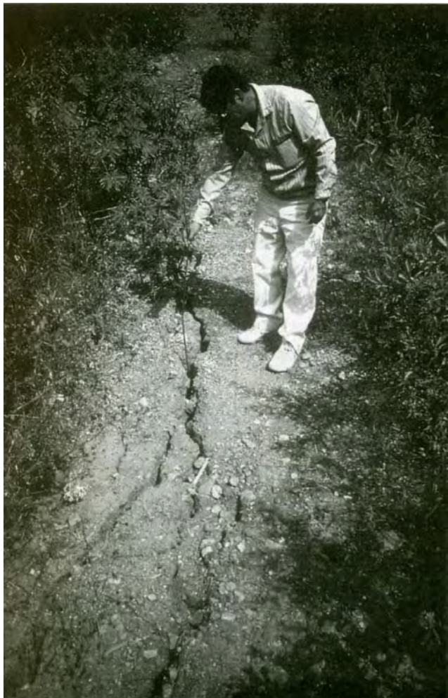
Photo 2.1 Tension cracks along a slope
