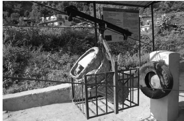
Photo 4: Example of a typical ropeway trolley
