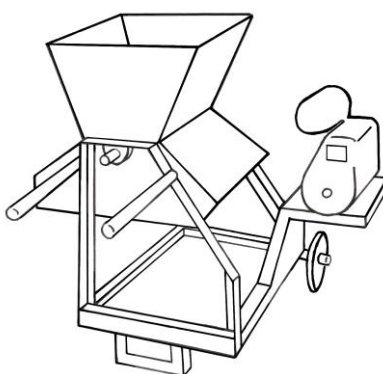
Figure 3: A cassava chipper Illustration: Neil Noble/Practical Action
