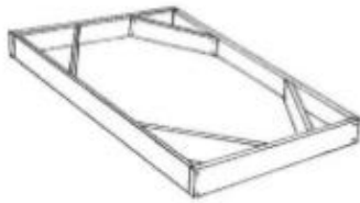
Figure 5: An alternative method of moulding using forms
