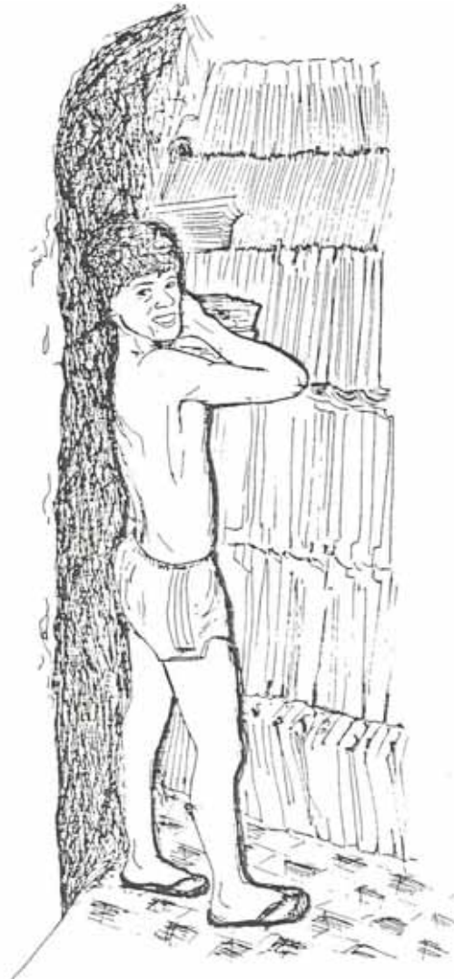
Figure 30: Stacking the tiles in the kiln.
