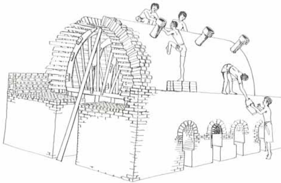
Figure 16: Kiln under construction showing roof mounted vent pipes made from ceramic gutter pipe
