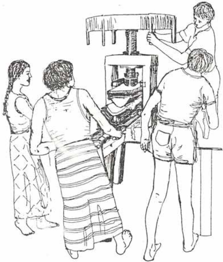
Figure 24: Pulling the lower die from the press.
