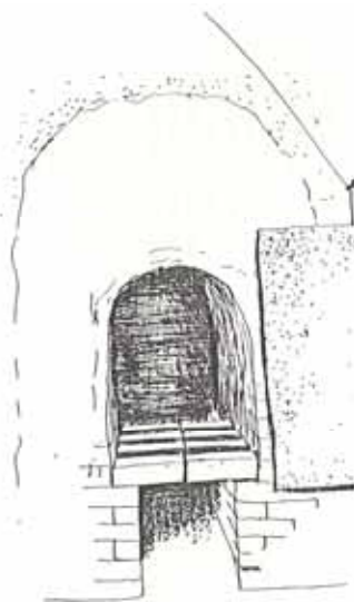
Figure 10: Kiln firebox fitted with butting brick grate arches.
