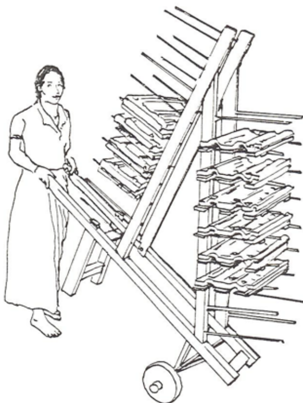
Figure 5: A cart for moving wet tiles.
