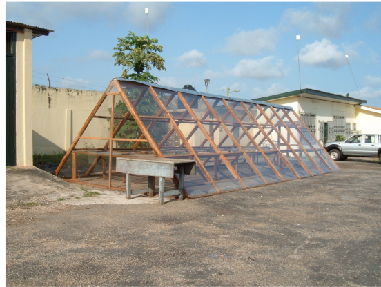
Figure 5: Large solar tent dryer, Ghana. Photo: Tony Swetman.
