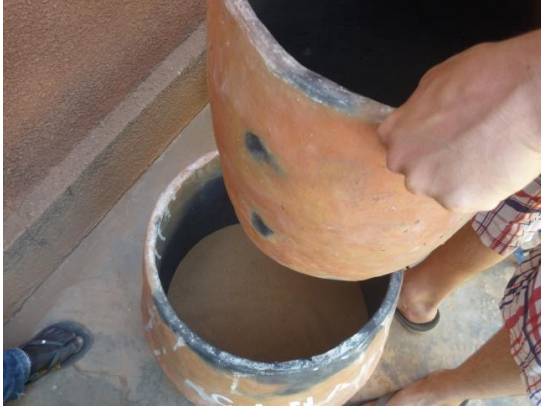
Figure 9: Smaller clay pot is placed in the bigger clay pot. Photo credit: Movement e.V. / Franziska Angermaier.
