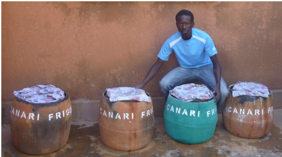
Figure 12: Movement team member with a test series of four covered clay pot coolers. Photo credit: Movement e.V. / Peter Rinker.
