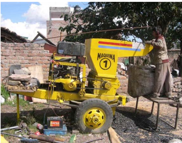
Photo 4: Shredder in Peru (Simone Ransijn)
