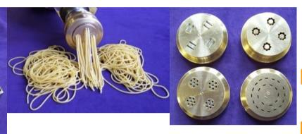
Figure. 1: Mixing pasta dough, extruded spaghetti, dies for pasta machines, pasta extruder, (Fords Food Equipment at www.freshpastamachines.co.uk/lillo due pasta machine.html)
