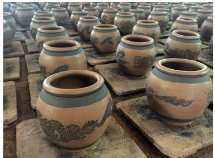
Figure 2: Raw earthenware “Dragon jars” at a factory in Ratchaburi, where the iron-rich soil gave the jars the right colours for the local market.
