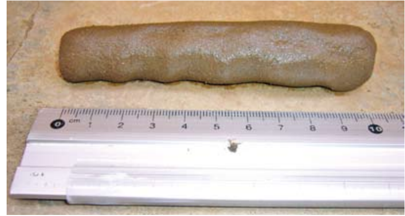
Pic 3. In this example the clay had shrunk to 93 mm a shrinkage rate of 7% which is acceptable
