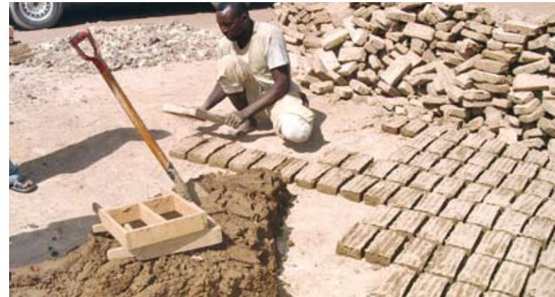
Pic 4. A participant using a moulding cast for brick production
