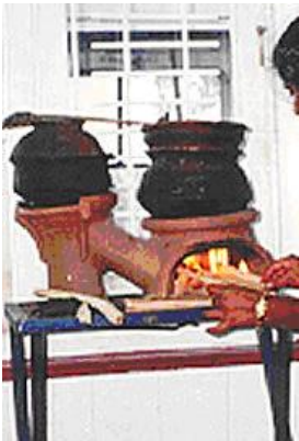
Stove type : Improved Construction material: Ceramic Chimney : no Fuel type : Wood Country : Sri Lanka
