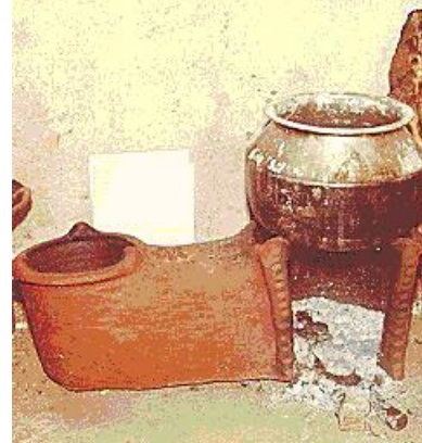
Stove type : Traditional Construction material: Ceramic Chimney : no Fuel type : Wood Country : Sri Lanka
