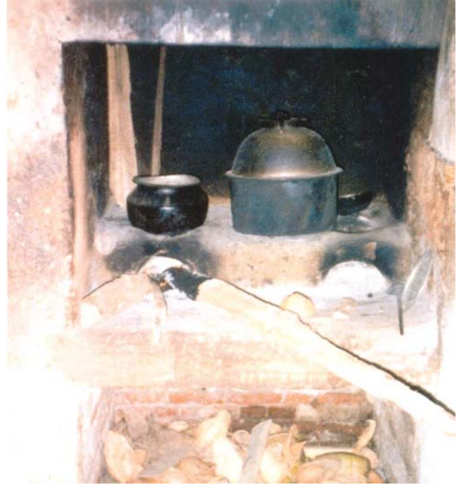
Biomass Stove for String Hopper Industry
