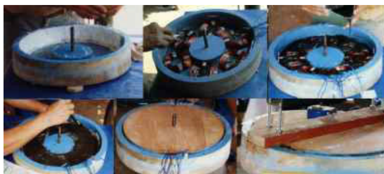
Six stages of the rotor casting procedure
