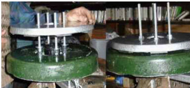
Fitting the front magnet rotor
