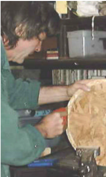
Sawing flat faces on the inner mould
