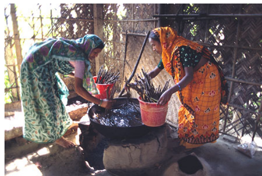
Figure 6: Zohrabanu & Amina boiling mulberry branches for pulp. Bangladesh. Photo: Zul / Practical Action.
