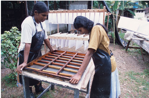
Figure 11: E D Karunawathi and Shanthi Dassanayake pressing to remove water. Photo: Zul / Practical Action.
