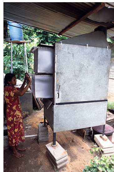
Figure 14: Indra Padmini loading paper into the dryer, (modified cashew dryer). Photo: Zul / Practical Action.
