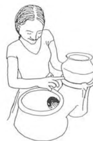
63. Use an aluminium pot to check that there is a very small gap above the shield. The pot should sit on the potrests, not on the shield.
