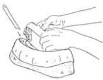
71. Cut excess clay along the same angle as the mould so the door will fit the firebox.
