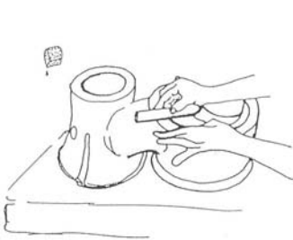
3. They are dampened with a sponge, and then rubbed with A wooden stick.
