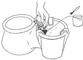
54. Score and slip the rim between the two potrests closest to the firebox.
