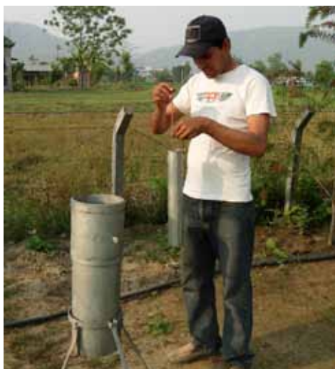
Photo 11: Measuring water by ruler.
