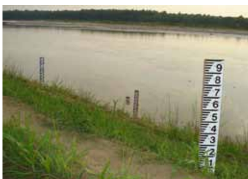
Photo 9: Water level gauges.
