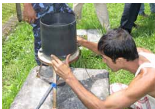
Photo 10: SEWIN_DHM_training-Automatic tipping bucket.
